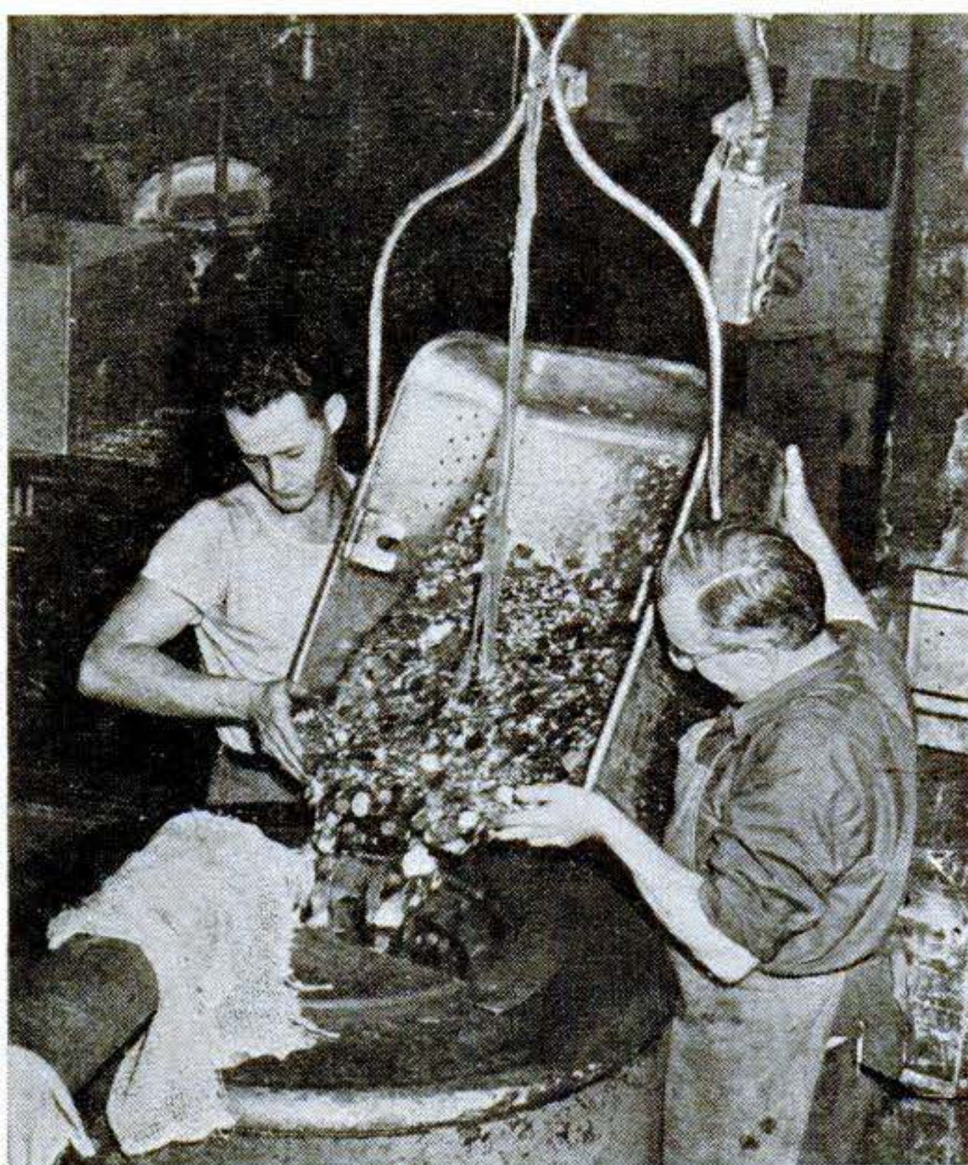
5. Emerging wet from a chemical cleaning solution, the blanks are dumped into this drier. A few whirls and they come out gleaming, looking like silver for the first time. From here they are fed into an "upsetting" machine that gives the blanks the raised rims. Precision again is paramount, for with uneven rims the finished coins would not stack properly.
